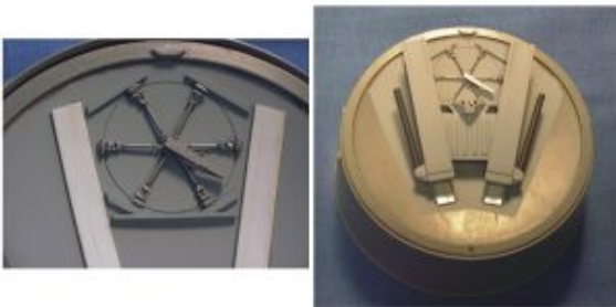
The finished LBP hatch and the rear bulkhead details.
